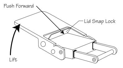
Some lid snaps have a lot of spring tension once they go over center, so keep a firm grip on the lid snap. Lid snaps may be opened one at a time or simultaneously.
